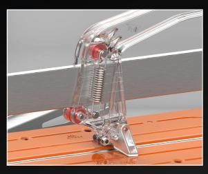
The carriage in aluminium is equipped with two ball-bearings one on the top and one on the bottom of the rail for a perfect sliding and top precision.
